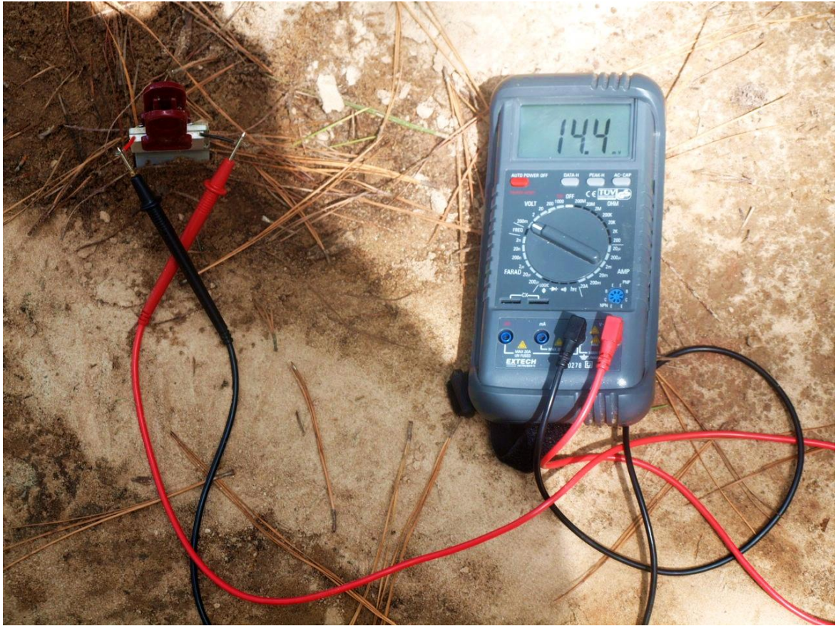
Figure 3.4: TEG on Aluminium plate giving above 10 mV
